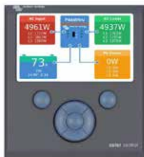
Color Control GX, showing a PV application
